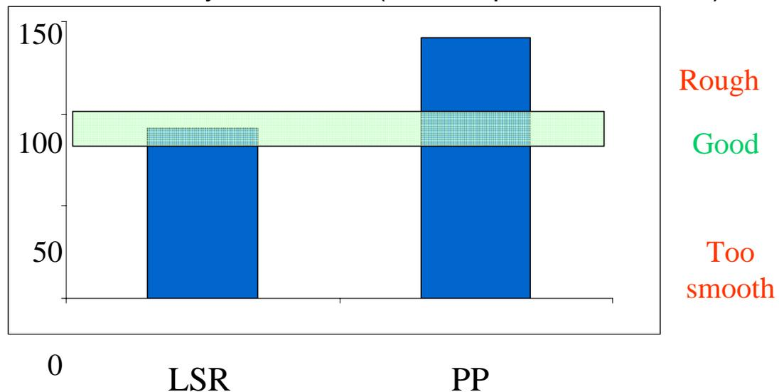
In the graph the Leroux tests done by Labosport France are shown. The Leroux value gives an indication of the field, whether it is good, too rough or too smooth. It is clearly shown that LSR<sup>®</sup> is positioned in the safe area.
