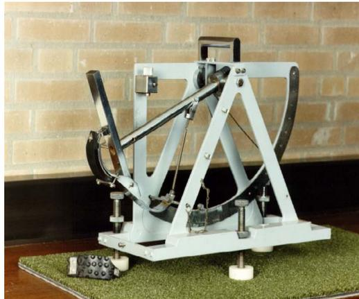
The underfoot friction is important for the players in order to reduce the risk of foot blocking during the foot-surface interaction. The method is different from the traction test, but it is measuring the same subject. Underfoot friction is obviously a measurement of the slipperiness of the surface and is measured using the Leroux machine as modified by NOC\*NSF (Dutch Sports Federation).
