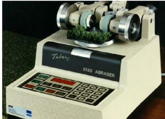
Fibres used in the sports surface industry must resist player and climate influences. One of the test methods available is the Taber test. In this test, two small, roughened wheels carry out a combined rolling/sliding movement across an artificial grass sample, indicating the wear resistance of the surface. This test can be done with both new and aged material, but is only useful for testing samples of water based pitches.
